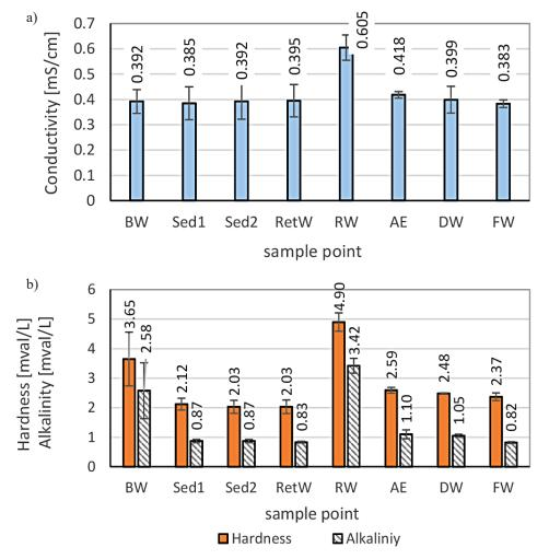
Fig. 2. Changes in the quality of water and recycled backwashings during treatment a) conductivity; b) hardness and alkalinity; c) pH and iron concentration; d) COD and turbidity
