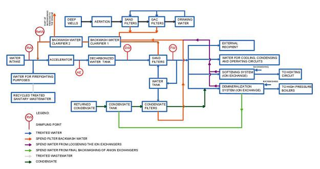
Fig. 1. Scheme of the WTP with recycled water streams and water sampling points
